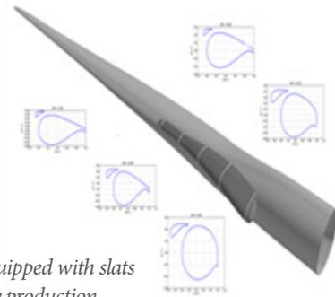
Figure 2 Blade equipped with slats to improve energy production
