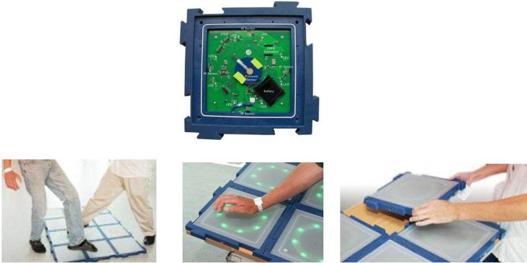
Figure 1: Modular tiles used for feet or hand interaction
