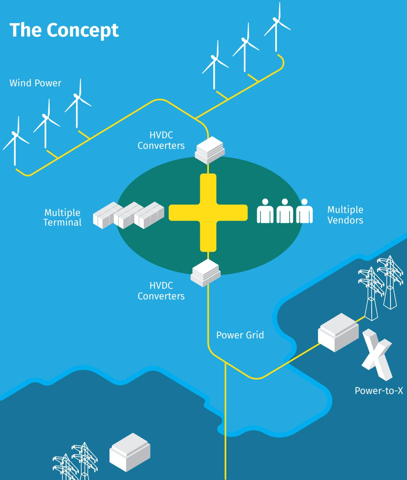
Energy islands are hubs connecting multiple offshore wind power plants to the power grid using multiple HVDC converters from different vendors. They may also host storage and power-to-gas conversion units.
